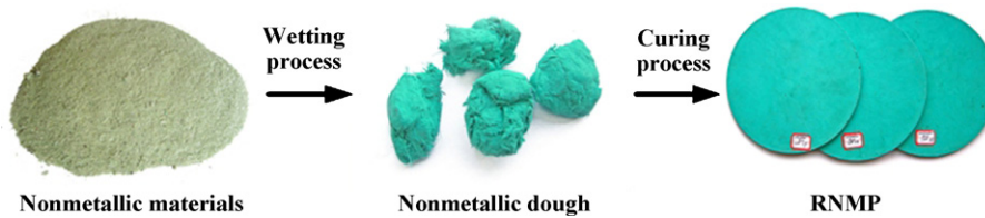
Fig. 4. Schematic illustration of production of RNMP.
